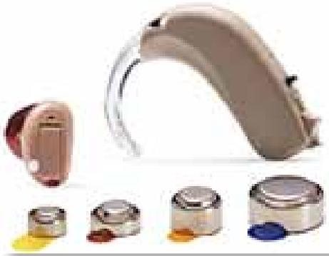
To optimize battery longevity, disengage it when the aid is out of use for a period of time. The most common period of regular disuse for most wearers is overnight. When the aid is removed at bedtime, the easiest thing to do is simply open the battery compartment door all the way and set the aid down on a dresser top or some other safe and convenient but accessible location.
